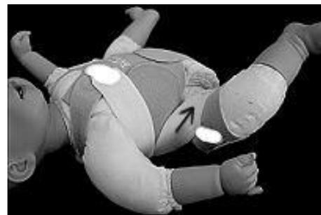
Fig. 32 Wrap the lower ends of the Cross Strap over the inner thigh and attach to the back of the limb cuff.
