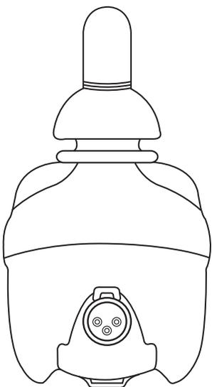
Plug the battery charger into the charging socket located at the front of the SHARK Control Unit.
