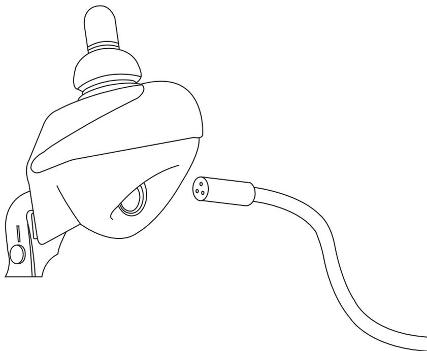
**WARNING: Do not exceed the maximum charging current of 12 A rms. Always use an off-board charger fitted with a Neutrik NC3MX plug. Failure to observe these conditions could result in poor contact resistance in the charger connector resulting in overheating of the charger plugs. This presents a potential burn hazard for the user. Penny & Giles accepts no liability for losses of any kind rising from the failure to comply with this condition.**
